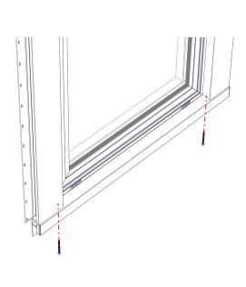
Add one  $\#8 \times 2$ " screw thru sill nose into the jamb casing on each end of sill nose.
