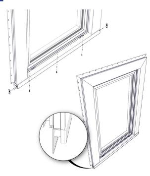
Install both sill nose end caps and attach the sill nose with #6 x  $\frac{1}{2}$ " pan head screws on the inside of window. Place screws 2" from each corner and 12" to 16" on center.
