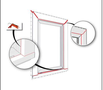
Apply a cap bead of sealant along all edges and corner where the WBMC meets the window.
